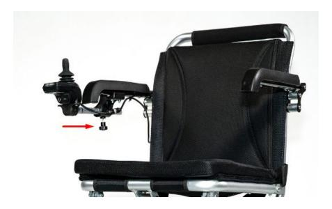
**Manual-Electric drive conversion** Lock the brake and turn off the power; pull the clutch (with red switch) out of the slot and turn right or left, make sure the clutch will not fall into the slot it is manual drive mode. Pull and turn the clutch again and make the clutch fall into the slot. It is electric drive mode.
