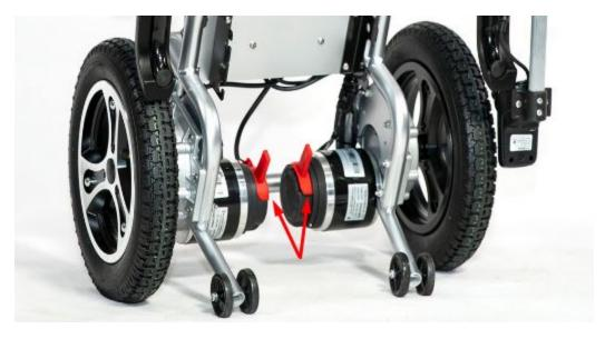
**Caution** When changing into electric drive mode, make sure both the left and right clutches are in the slot. If any side of the clutch can not completely fall into the slot, there will be danger of side-turning over
